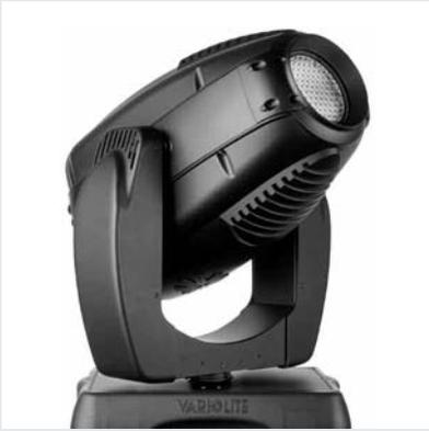
The VARI\*LITE® VL3000™ Wash luminaire features 6:1 zoomable beam spreader optics, CYM color mixing, variable CTO color temperature correction, a six-position color wheel and separate dimmer and ultra-fast strobe mechanisms. A standard palette of colors is provided with the unit. Custom colors are available.
